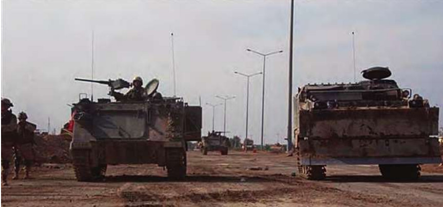
An M113 armored personnel carrier and an M9 armored combat earthmover of the 2d Platoon, Company A, 82d Engineer Battalion, on a road near Fallujah. The unit's M9s were instrumental in breaching the city's outer ring of defenses at the beginning of the battle.
