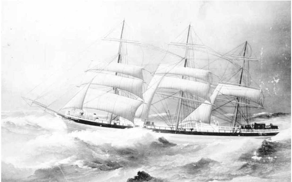
The SEEADLER in her previous incarnation as the PASS OF BALMAHA. The removal of her upper or royal yards (a money-saving measure) gave her spars a somewhat foreshortened look.
