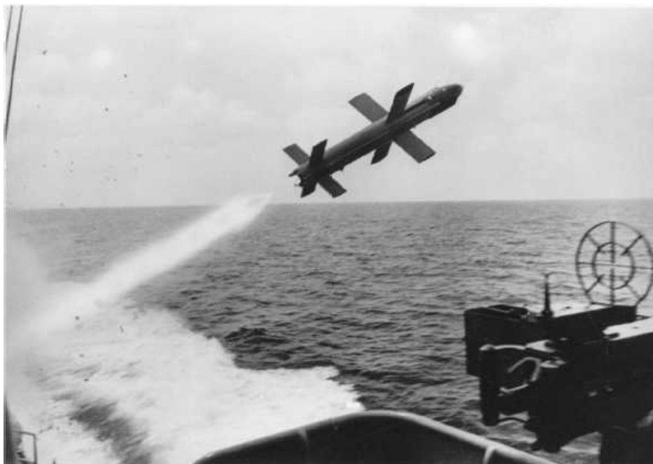
A Gabriel lifts from the deck of an Israeli missile boat. After arcing upward, it will dive and skim over the surface of the sea to its target.
