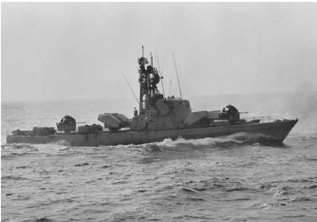
A missile boat with guns and missile launchers fore and aft and a mast bristling with electronics devices is little bigger than a conventional patrol boat but has the punch of a major warship.
