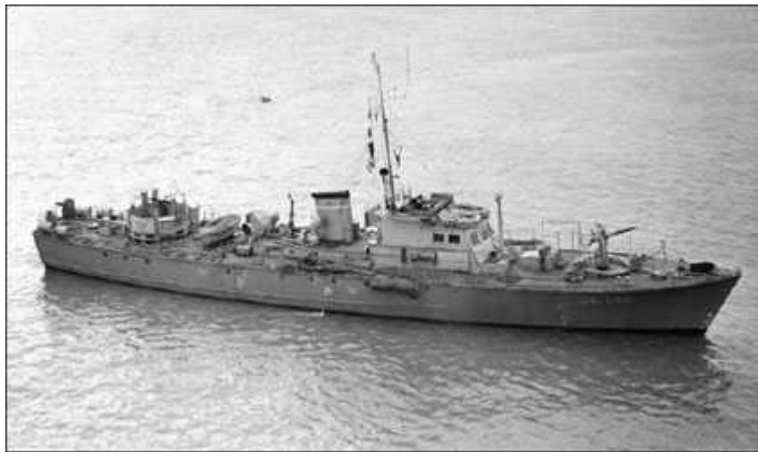
Fairmile 'B' Class launch, the most numerous of the small vessels used in the raid. This illustration shows the type of motor launch, but not one that actually took part in the St Nazaire operation. Its forward armament is a 3-pdr Hotchkiss, whilst aft is a 20mm Oerlikon. On the bridge are two twin Lewis .303in. machine-guns.
