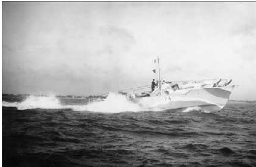
Lt Wynn's MTB 74 at speed. The two massive high-mounted torpedo tubes give the boat a powerful profile. Capable of almost 40 knots, it was easily the fastest craft on the raid.
