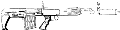
Preproduction models with different butts and pistol grips. The foregrip differs from the production model.
